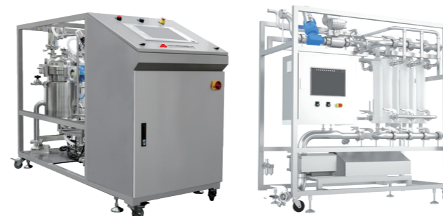
Figure 10: Industrial scale automatic tangential flow filtration system
