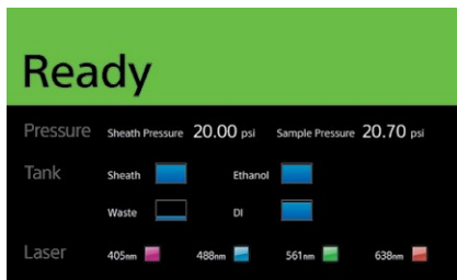
The LCD monitor on the front of the SH800S displays status information during operation.
